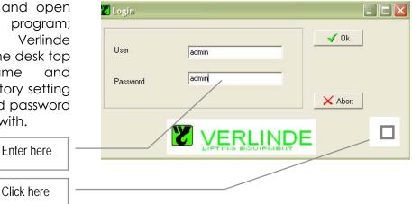
Click on the **D** box to confirm that good notice is taken of all *"Notes on Safety"* as mentioned in the hoist and controller manual. The start up procedure won't proceed if this confirmation is not made.
