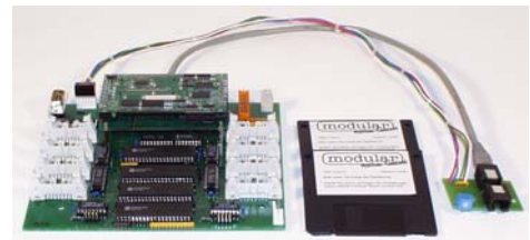
Processor board to transform a R8PRM-C1 into a R8CPU-C1.
