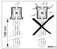
**Note:** Make sure that the stop is correctly fitted. The locking tube should be turned towards the hoist.
