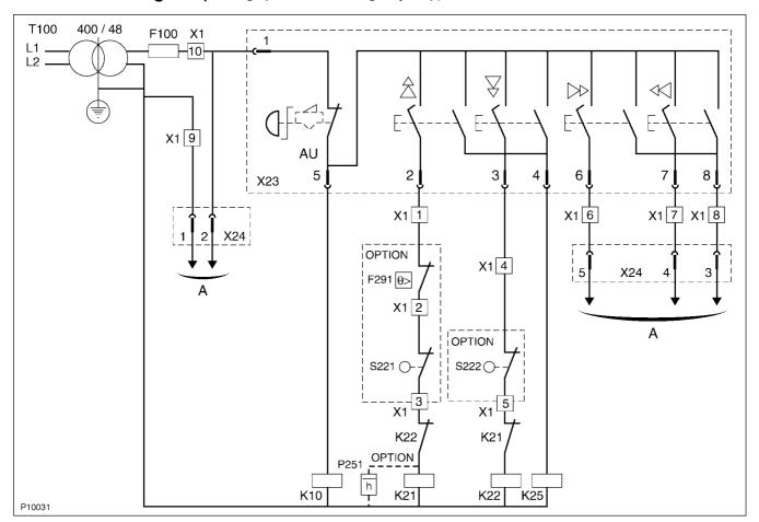
Electric trolley Α ΑU Emergency stop T100 Control transformer F100 T 1,25 A fuse K10 Emergency stop control K21 Lifting control Lowering control Speed selector K22 K25 X1 Hoist terminal
