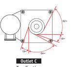
Top fixation Rope fixed on the gear side
