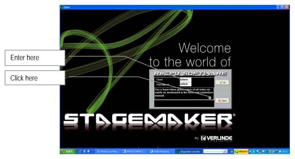
Click on the box to confirm that good notice is taken of all "Notes on Salety" as mentioned in the Hoist and controller manual. The start up procedure won't proceed if this confirmation is not made.
