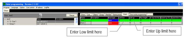
These given values might be subject of change as they are depending on type of mechanical limit switch applied. A proper setting is essential in order to avoid interference of these safety devices during normal operations. The operational software limit could be set at any convenient position with a minimum of 0.1m from the Max. Height position.
