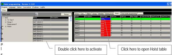
Complete the list by entering the software limits for Up and Down as well as for the safety limit Max. Height related to the Show location. Keep in mind that the Hoist has also a mechanical safety limit switch that should be adjusted with the lifting hook for Upper position as well as the chain stopper for Lower position at minimum 0.2m from the Hoist body. The "Max. Height" setting is an additional safety limit and should be set between upper limit switch level and upper software limit.
