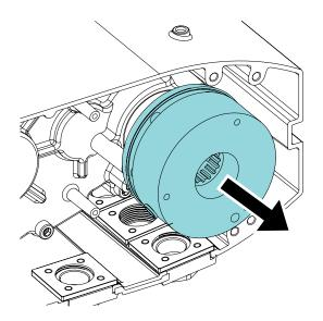
8. Install the new brake on the shaft.
