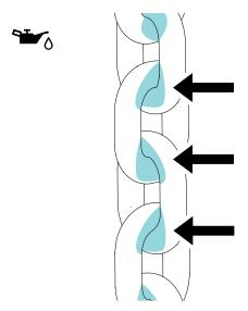
Figure 19. Correct lubrication points on the chain
