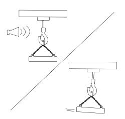
3. Press the DOWN push button to lower the load.
