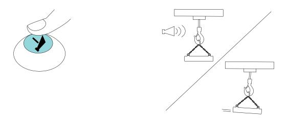
3. Press the push button UP gently to take up the slack from the chains or sling slowly before lifting the load from the ground.
