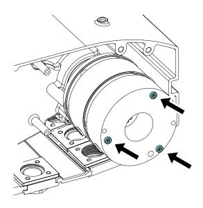
10. Remove the brake carefully.
