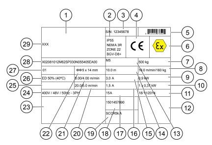
Figure 1. CE data plate for chain hoist
