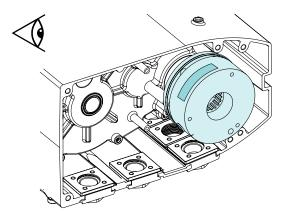
5. Unplug the brake cable (1) from the control board.
