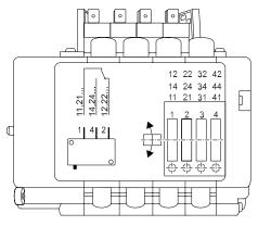
Figure 15. 4-step rotating geared limit switch
