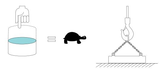
4. Continue to press the push button UP until the load is barely clear of the ground.
