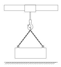
• Chain hoist must be positioned directly above (perpendicular to) the load so that there are no side-pulling forces.
