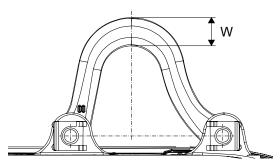
Figure 17. Measuring wear on the suspension bracket (option)
