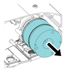
11. Assemble the new double brake.
