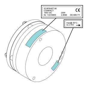
The brake wear value varies according to the brake manufacturer and brake series. For each brake type, the maximum value for the wear is indicated on the brake data sticker on the brake.
