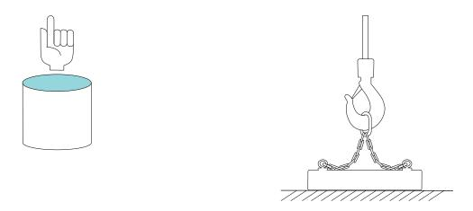
2. If the hoist has an alarm horn, press the alarm horn push button to warn people nearby that a load is about to be moved.
