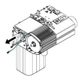
14. Plug in the brake cables (1) and (2).
