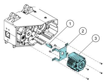
Figure 8. 4-step rotating geared limit switch
