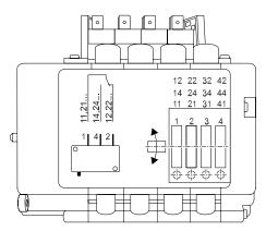
Figure 10. 4-step rotating geared limit switch
