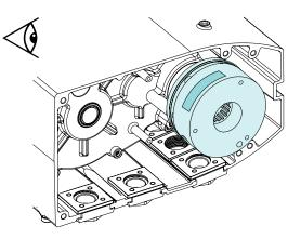
5. Unplug the brake cables (1) and (2) from the control board.
