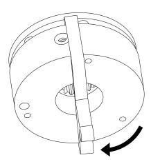
3. Tilt the manual brake release lever in the brake gap. Press the lever carefully to open the brake.
