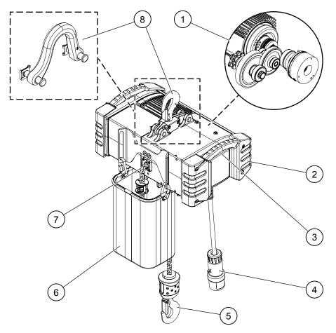
Figure 7. Main components of the electrical chain hoist
