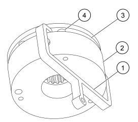
2. Turn the manual brake release lever so that its second arm fits into the brake gap on the opposite side of the brake.
