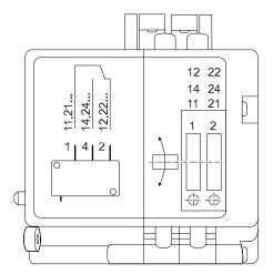
Figure 14. 2-step rotating geared limit switch
