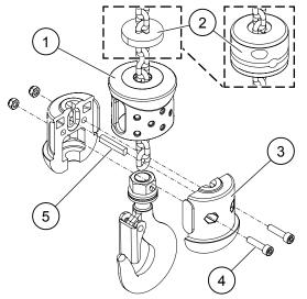
8. Pull the rubber plate or the limit switch activator up on the chain. Attach the end stop to the chain end on the chain bucket side of the chain fall.
