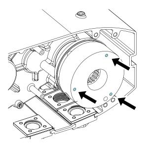
10. Remove the brake carefully.
