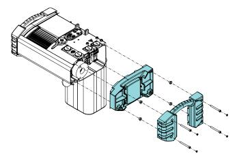
3. To access the components on the motor side, loosen the four screws of the end cover on the motor side. Remove the end cover.
