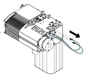
8. Check that the brake data of the replacement brake matches with the data of the original brake.
