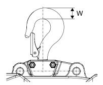
Figure 16. Measuring wear on the rotating suspension hook
