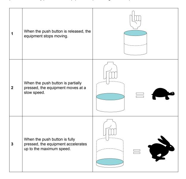
NOTE If you press a push button (for example hoist UP) while the opposite direction push button is pressed (for example hoist DOWN), the lifting device does not change direction.
