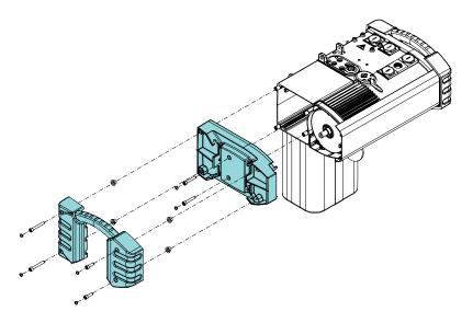
4. To install the end covers, put the end cover back on its place on the hoist frame. Tighten the fours screws to the correct tightening torque.
