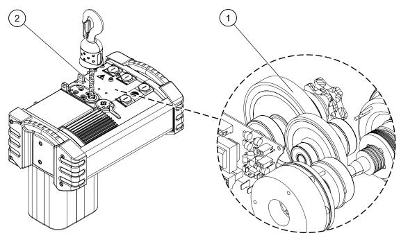
Figure 23. Lubrication points of the chain hoist
