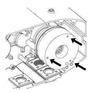
7. Remove the brake carefully.
