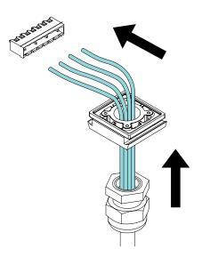
3. Slide the power supply cable assembly in place. Connect the power supply plug to the power supply socket.
