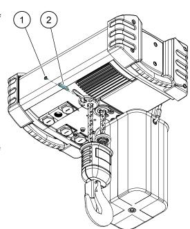
Pull the rubber buffer up on the chain.
