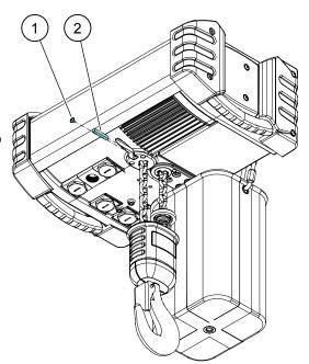
5. Remove the hook and the hook block by pulling the chain out through the hook block.
