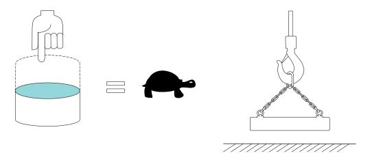
5. Fully release the DOWN push button when there is slack in the lifting device but before the hook or lifting device impacts the load.
