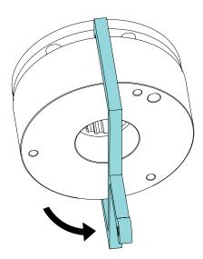
4. Repeat the procedures for pressing the lever and lowering the load within short intervals.
