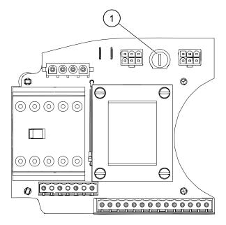
Figure 18. Power supply board with control voltage fuse
