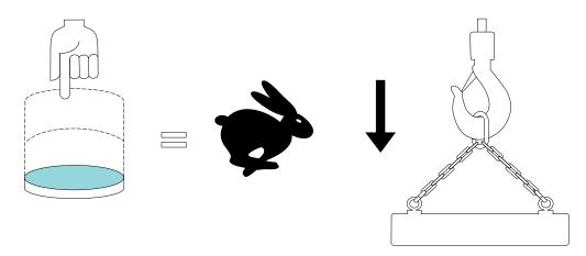
4. Decrease the lowering speed by gradually releasing the DOWN push button when the load approaches the ground.
