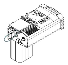
6. Remove the end cover on the brake side. For more information, see chapter Removing and installing the hoist covers.
