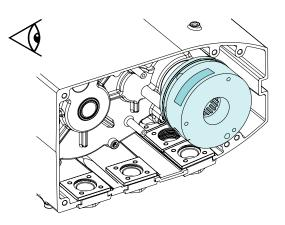
9. Remove the three screws that hold the brake in place.
