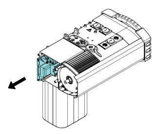
When the control board is a few centimeters out, unplug the brake cables
