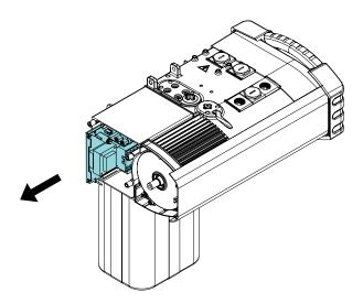
When the control board is a few centimeters out, unplug the brake cable (1) from the control board.
