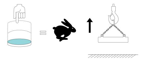
6. Release the UP push button gently when the load is at the desired height. Do not raise the load higher than is necessary to avoid colliding with objects.
