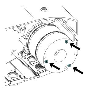
7. Remove the brake carefully.
