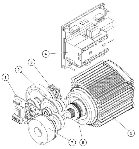
Figure 6. Main components of the lifting function
