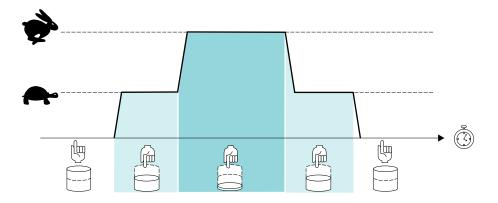
The motor runs at one of two preset speeds corresponding to the force that the operator applies to the direction control push button. When you press the direction control push button half-way down, the motor runs at its slowest speed. When you press the direction control push button fully down, the motor runs at its maximum speed. When you release the direction control push button, the motor stops running.
