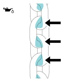
Figure 21. Well lubricated chain
