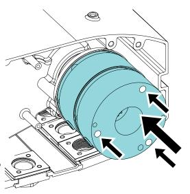
13. Lead the brake cables through the hoist frame. Pull the brake cables carefully out on the motor side.
