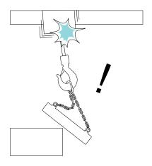
• If the load is unstable, it can exert a sudden force on the chain. Fasten the contents of the packing cases securely, so that they cannot move around during lifting.
