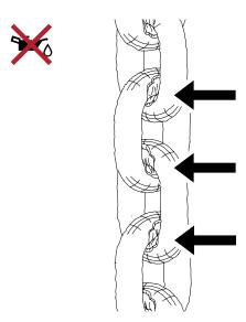
Figure 22. Completely dry and damaged chain
