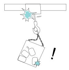
• Sudden loss of the load can cause the trolley or hoist to jump.
