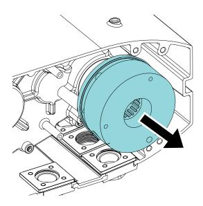
11. Install the new brake on the shaft.
