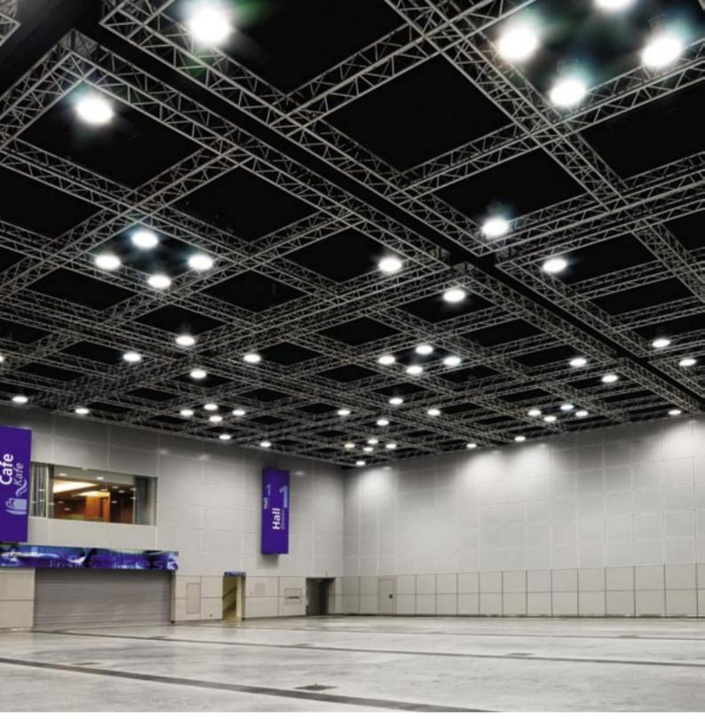
Above: Inside the Exhibition Hall, the motorised grid ceiling from VME Material Handling is a distinctive architectural feature. Designed and made locally, each section of the grid was created at VME's factory and then assembled on site. Installation took six weeks and was completed ahead of time.
