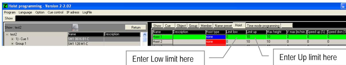
These given values might be subject of change as they are depending on type of mechanical limit switch applied. A proper setting is essential in order to avoid interference of these safety devices during normal operations. The operational software limit could be set at any convenient position with a minimum of 0.1m from the Max. Height position.
