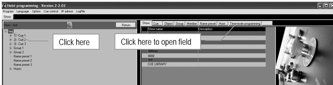
2) Enter a reference or give the effect a name in the Title field. Double click in the column Synchro to activate Yes for synchronised operations in time mode, or No for non synchronised operations in fixed speed mode. The option Yes for time based operations is not available in case of Hoists with fixed speed. Select Manual or Automatic in the last column Cue connect, if the next Cue in sequence start after manual command or automatically.
