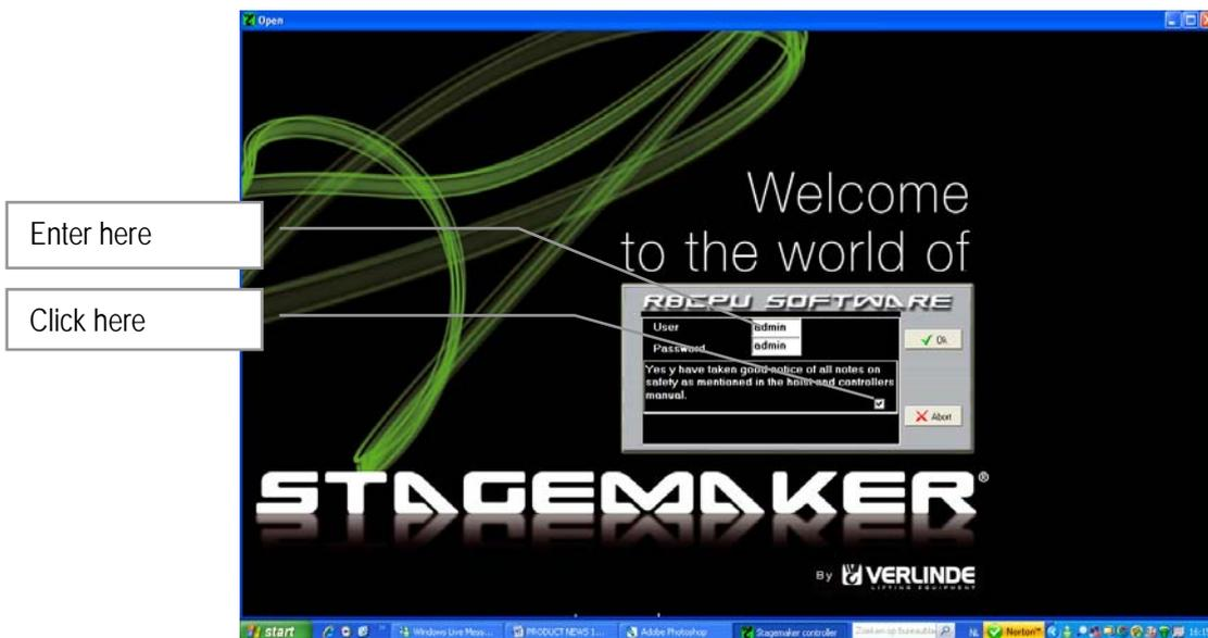
Click on the  box to confirm that good notice is taken of all "Notes on Safety" as mentioned in the Hoist and controller manual. The start up procedure won't proceed if this confirmation is not made.
