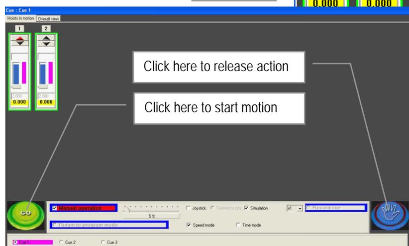
15. Use the Joy-stick to select the speed suitable for the operation of that moment. Adapt the speed to the operating circumstances pressing the stick more or less forward whilst pressing the ● dead mans button or the little button on top of the joy-stick. This option is only effective in combination with variable speed Hoists
