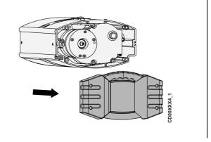
Open the brake side cover. Pull the brake cables with the brake plugs carefully out on the brake side.
