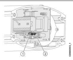
When the electrical board is a few centimeters (inches) out, unplug the brake plugs (1) and (2) from their sockets.
