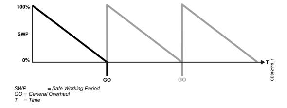
Once the SWP% of the hoisting machinery reaches zero, the hoisting machinery has exhausted its theoretical lifetime. The probability of a defect in the product is therefore higher and operating safety is jeopardized. At the end of the SWP, a thorough General Overhaul (GO) must be conducted. Afterwards the product will then be assigned a new SWP, provided that it is safe to continue operation. At the start of each period the SWP is 100% and, at the end, the SWP is 0%.
