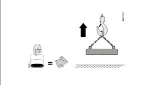
Check, at fast speed, the lifting of a nominal load.
