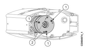
Tighten the screws (1) with a tool. Remove the two other screws (2).
