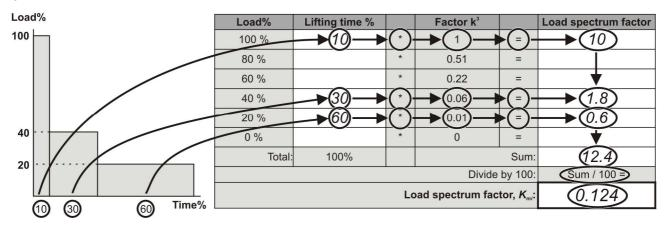
Step 3: Calculate the partial duration of service, S<sub>i</sub>
