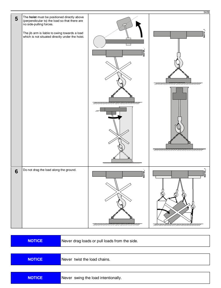
The operator shall ensure that the hoist or the load does not collide with anything or fall from the lifting device.
