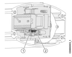
Plug the brake plugs on their correct sockets.
