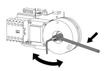
Turn the screw clockwise to increase the torque, counterclockwise to decrease the torque. Unscrew the nut to adjust the setting with the screw and tighten the nut to lock the setting when it's correct.
