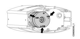
Unscrew the three screws of the brake.
