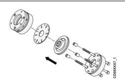
Assemble the brake according to the picture.
