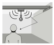
Hoists generate some audible noise during operation. The total noise level experienced in the operating area is a combination of the individual noise sources around the operator. The main sources of noise from the hoist arise from its components, vibrating structures and reflective surfaces.
