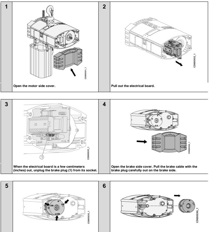
Remove the brake by pulling it out.
