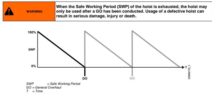
Once the SWP% of the hoisting machinery reaches zero, the hoisting machinery has exhausted its theoretical lifetime. The probability of a defect in the product is therefore higher and operating safety is jeopardized. At the end of the SWP, a thorough General Overhaul (GO) must be conducted. Afterwards the product will then be assigned a new SWP, provided that it is safe to continue operation. At the start of each period the SWP is 100% and, at the end, the SWP is 0%.
