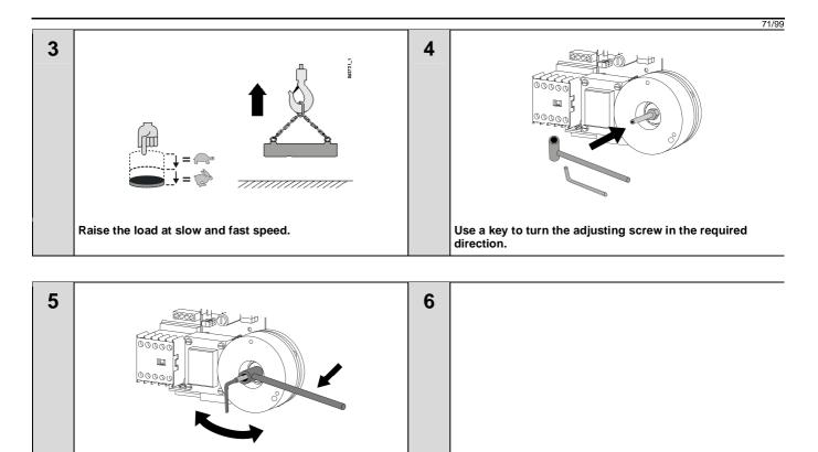
Turn the screw clockwise to increase the torque, counterclockwise to decrease the torque. Unscrew the nut to adjust the setting with the screw and tighten the nut to lock the setting when it's correct.
