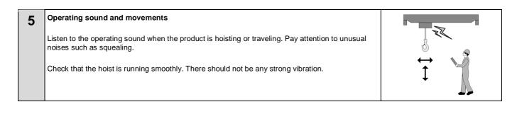
Any defects or abnormalities which are detected during the commissioning must be investigated and corrected in accordance with the instructions relevant to the component in question.
